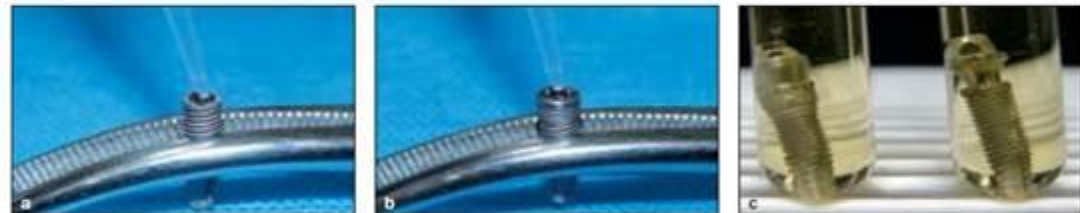
Fig 2 (a and b) Inoculation of S aureus into the internal part of the implants; (c) assemblies submerged in BHI broth.
